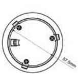
Recessed: Cut out size: Ø59-60mm
