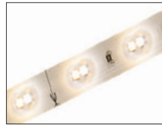
Cool white and warm white diodes side by side creating natural white
